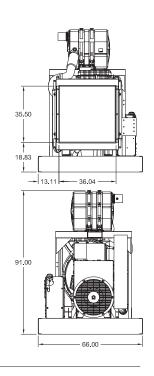
Drawings based on standard open power 480 volt standby generator. Lengths may vary with other voltages. Subject to change without notice. Sound data as measured at 23 feet (7 meters) in accordance with ISO 8528-10 at standby rating.
